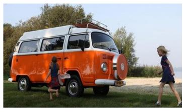
Aesthetically, it hasn't changed too much from its days as transport for Kiwis on their OE. But the van's air-cooled flat fourcylinder engine has been replaced with a more modern 1.4-litre inline four, and the "spare tyre" on the front is actually an air filter that hides a front-mounted radiator.
